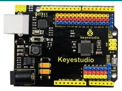
This board has an ATMEGA16U2 chip which can be UART-to-USB conversion plug.
