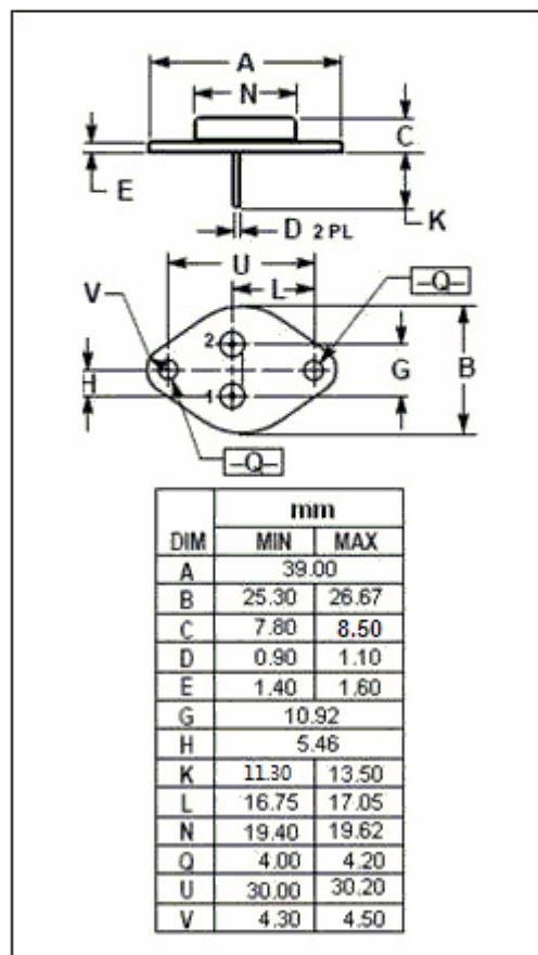
**isc Silicon NPN Power Transistor****ISC53****ELECTRICAL CHARACTERISTICS**T<sub>c</sub>=25°C unless otherwise specified
