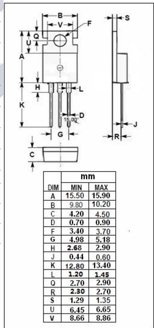
**isc N-Channel MOSFET Transistor****IRFZ24N****ELECTRICAL CHARACTERISTICS****T<sub>c</sub>=25°C unless otherwise specified**
