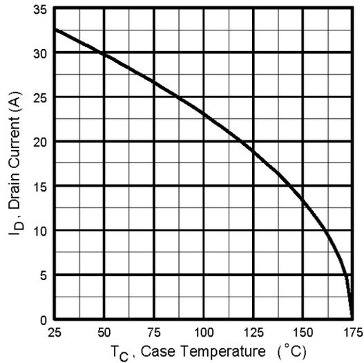
**Fig 9.** Maximum Drain Current Vs. Case Temperature
