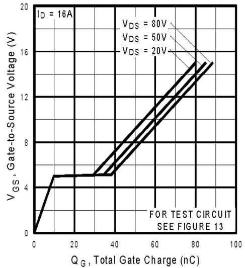
**Fig 6.** Typical Gate Charge Vs. Gate-to-Source Voltage
