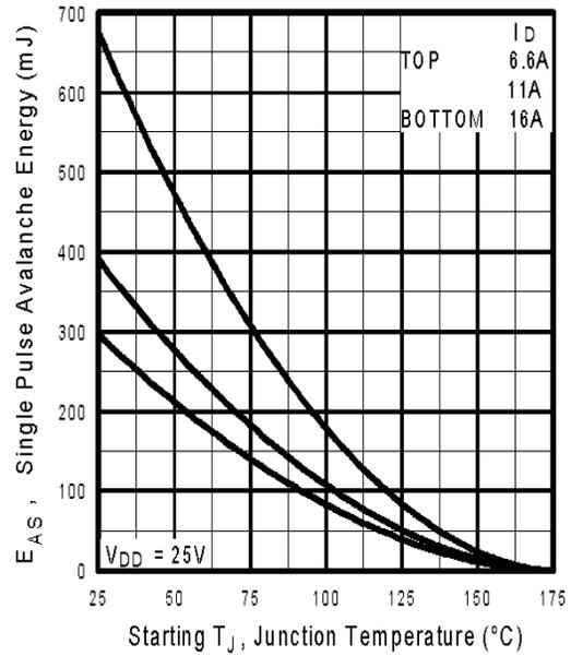
**Fig 12c.** Maximum Avalanche Energy Vs. Drain Current
