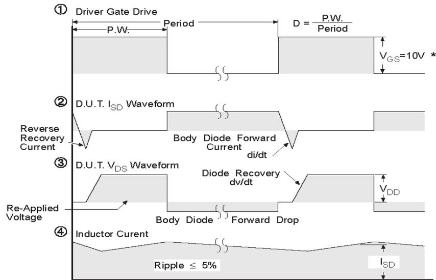
\*  $V_{GS} = 5V$  for Logic Level Devices
