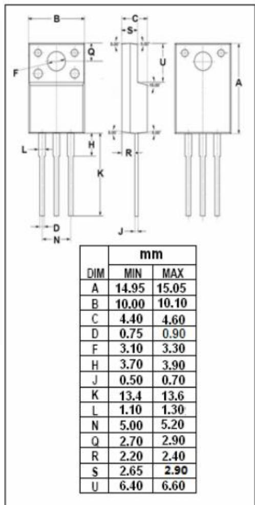
**isc N-Channel MOSFET Transistor****IRFI540N, IIRFI540N****ELECTRICAL CHARACTERISTICS** $T_c=25^\circ\text{C}$  unless otherwise specified
