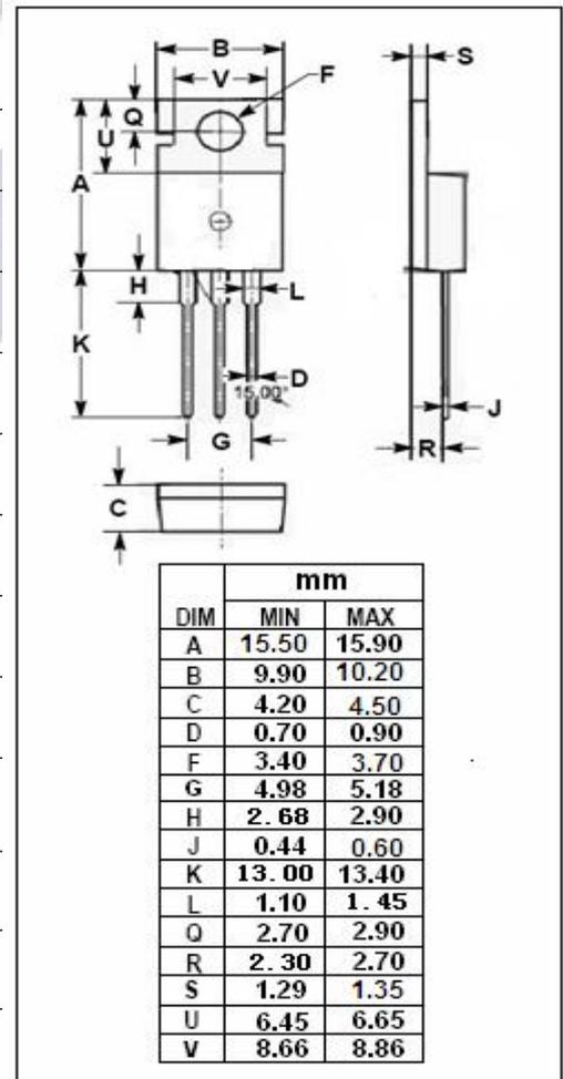
**isc N-Channel MOSFET Transistor      IRFB23N15D, IIRFB23N15D**
