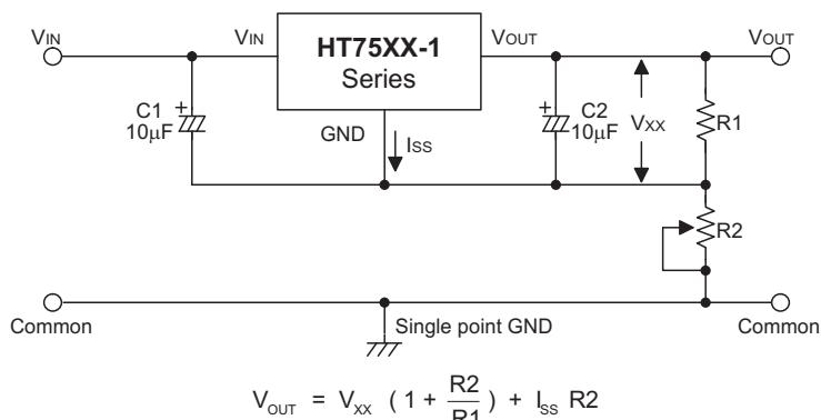
**Circuit for Increasing Output Voltage**
