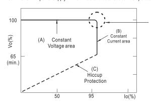
Typical LED power supply I-V curve
