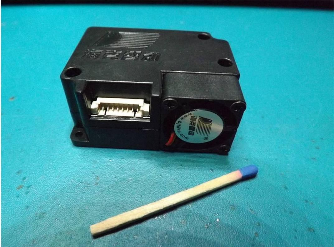
Fig. 2: Fan (air outlet) and connector
