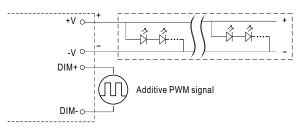
"DO NOT connect "DIM- to -V"
