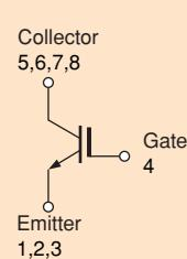
All the emitter terminals should be connected together.
