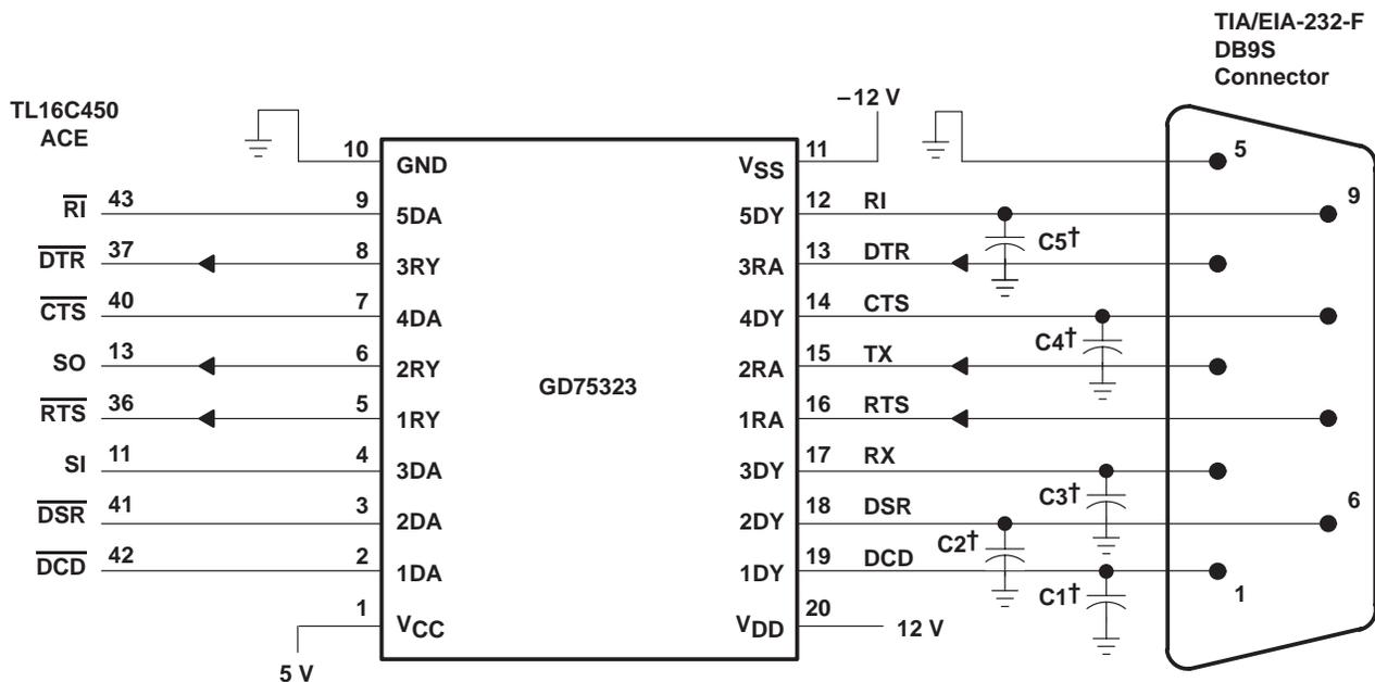
† See Figure 10 to select the correct values for the loading capacitors (C1, C2, C3, C4, and C5), which may be required to meet the RS-232 maximum slew-rate requirement of 30 V/μs. The value of the loading capacitors required depends upon the line length and desired slew rate, but is typically 330 pF.
