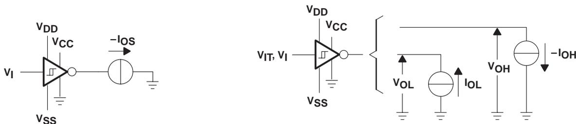
Figure 4. Receiver Test Circuit for  $I_{OS}$
