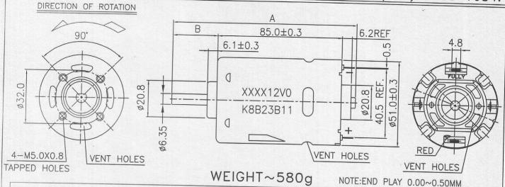
LENGTH OF SHAFT (A): 120.0 MM (±0.1) FRONT EXTENSION (B): 27.0 MM (±0.5)
