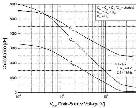
Figure 5. Capacitance Characteristics
