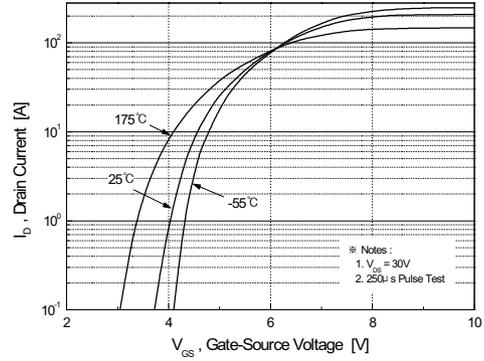
Figure 2. Transfer Characteristics
