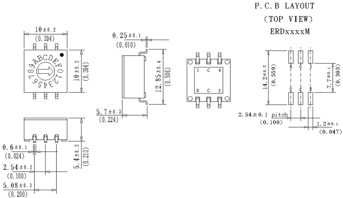
**DIMENSIONS AND CIRCUITRY UNIT:mm(inch) PIN OUT 1:4**
