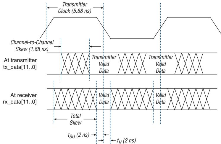
Table 5–48 shows the mini-LVDS transmitter timing budget for Cyclone II devices at 311 Mbps. Cyclone II devices can not receive mini-LVDS data because the devices are intended for applications where they will be driving display drivers. A maximum mini-LVDS data rate of 311 Mbps is supported for Cyclone II devices using DDIO registers. Cyclone II devices support mini-LVDS only in the commercial temperature range.
