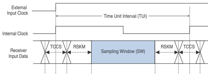
Figure 5–4 shows the high-speed I/O timing budget.
