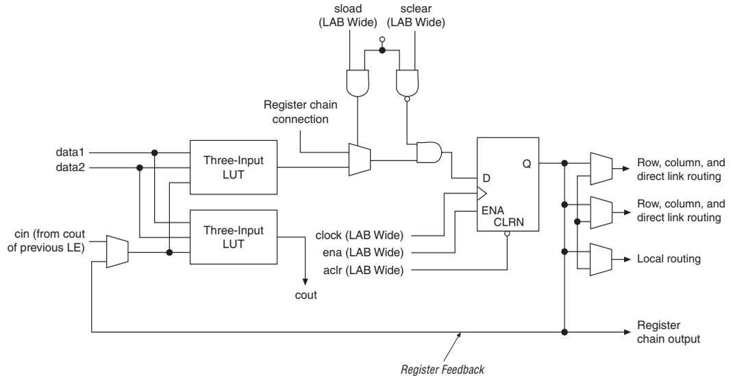
The Quartus II Compiler automatically creates carry chain logic during design processing, or you can create it manually during design entry. Parameterized functions such as LPM functions automatically take advantage of carry chains for the appropriate functions.
