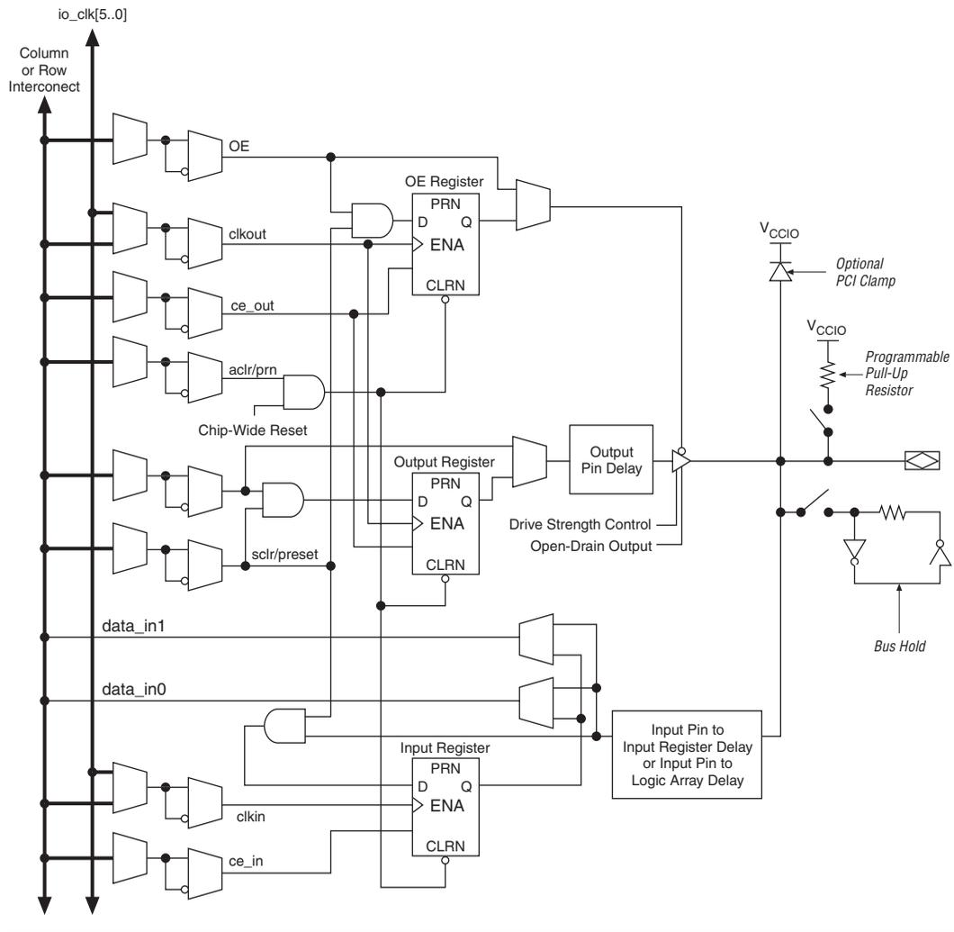
The Cyclone II device IOE includes programmable delays to ensure zero hold times, minimize setup times, or increase clock to output times.
