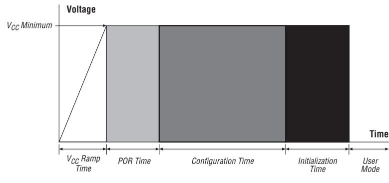
The  $V_{CC}$  ramp time and POR time will depend on the device characteristics and the power supply used in your system. The fast-on devices require a maximum  $V_{CC}$  ramp time of 2 ms and have a maximum POR time of 12 ms. (The values for maximum  $V_{CC}$  ramp time and maximum POR time for the fast-on devices are preliminary. Altera will provide a final value upon completion of characterization of the fast-on devices).
