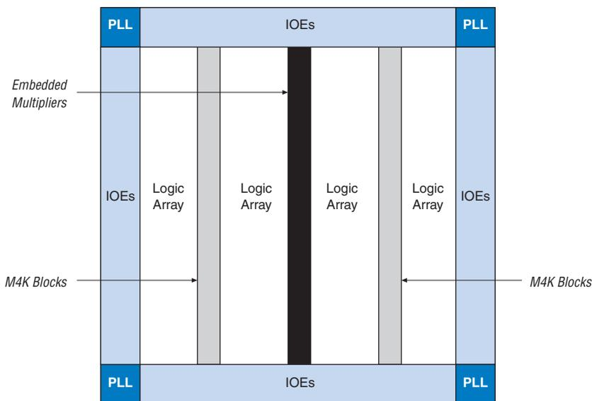
The number of M4K memory blocks, embedded multiplier blocks, PLLs, rows, and columns vary per device. Table 2–1 lists the resources available in each Cyclone II device.
