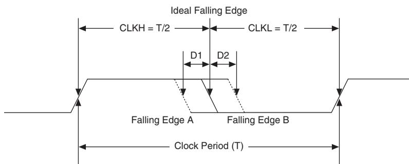
DCD expressed in absolute derivation, for example, D1 or D2 in Figure 5–8, is clock-period independent. DCD can also be expressed as a percentage, and the percentage number is clock-period dependent. DCD as a percentage is defined as:
