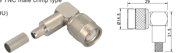
M57714 Right angle TNC male twist on type gold-pin (RG58U/59U)
