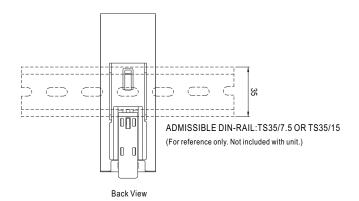
This series fits DIN-RAIL TS35/7.5 or TS35/15. For installation details, please refer to the USER MANUAL on http://www.meanwell.com/search/EDR-150/EDR\_manual.pdf
