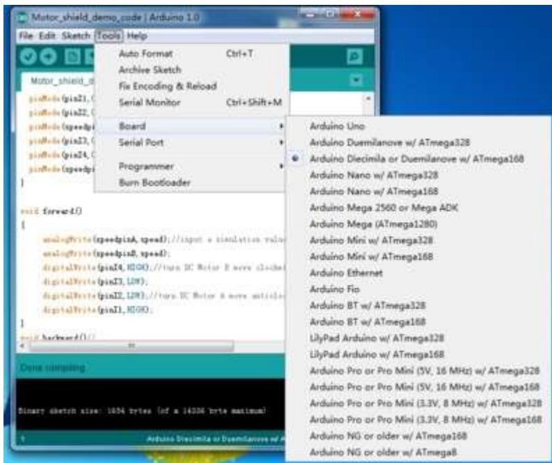
Upload the sketch to your Arduino board, then you would find the 2 motors begin to work. If you power the motor shield via the power terminal and the power jumper J4 was inserted, you can remove the USB cable now. Speed control is achieved through conventional PWM which can be obtained from Arduino's PWM output D9(EA) and D10(EB). Using the function `analogWrite()` to generate the drive PWM:
