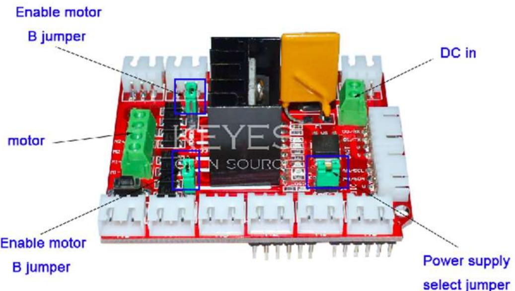
Enable Motor B jumper: Connect above two interfaces with a jumper cap when driving the DC motor A.
