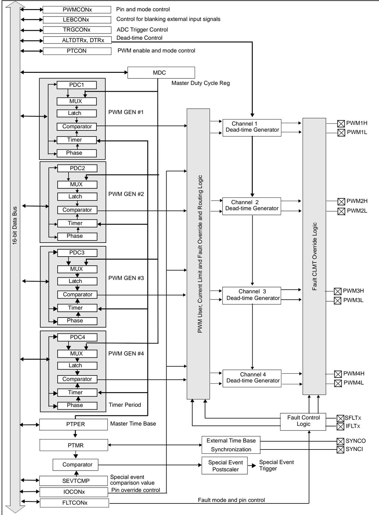
**FIGURE 12-2: PARTITIONED OUTPUT PAIR, COMPLEMENTARY PWM MODE**
