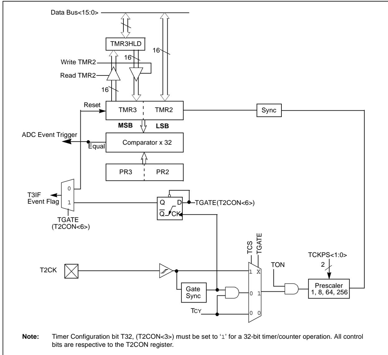
**FIGURE 9-2: 16-BIT TIMER2 BLOCK DIAGRAM**
