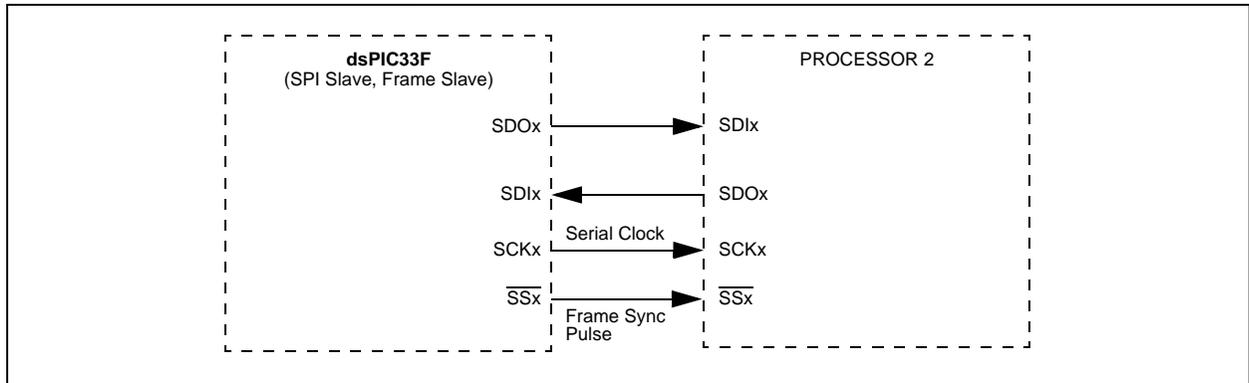
**FIGURE 13-4: SPI MASTER, FRAME SLAVE CONNECTION DIAGRAM**
