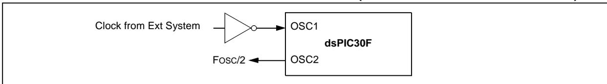
**FIGURE 18-5: EXTERNAL CLOCK INPUT OPERATION (ECIO OSCILLATOR CONFIGURATION)**
