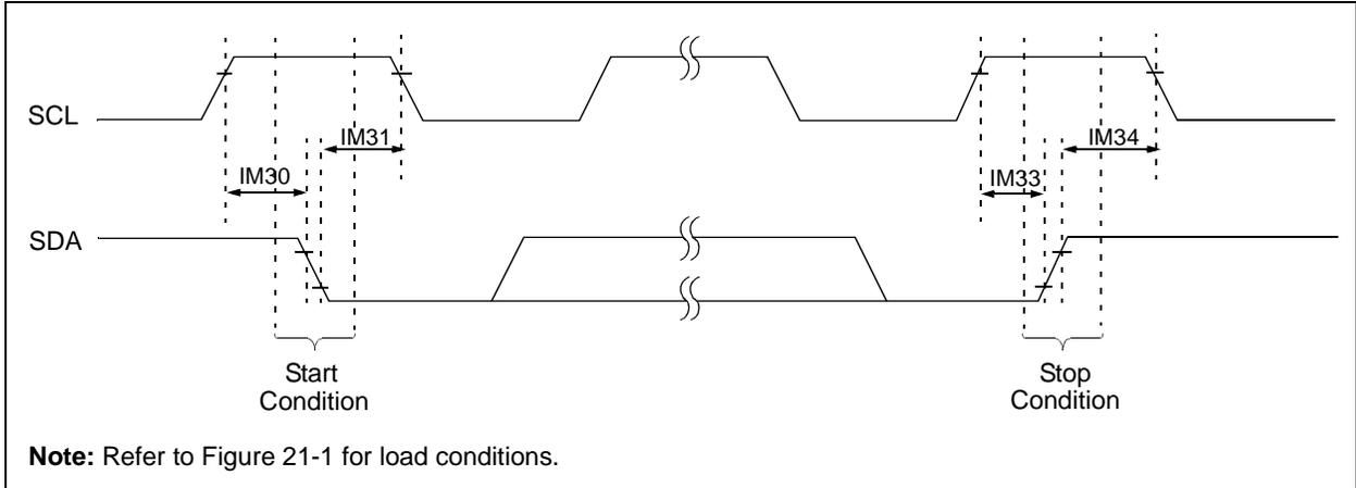
**FIGURE 21-17: I<sup>2</sup>C™ BUS DATA TIMING CHARACTERISTICS (MASTER MODE)**
