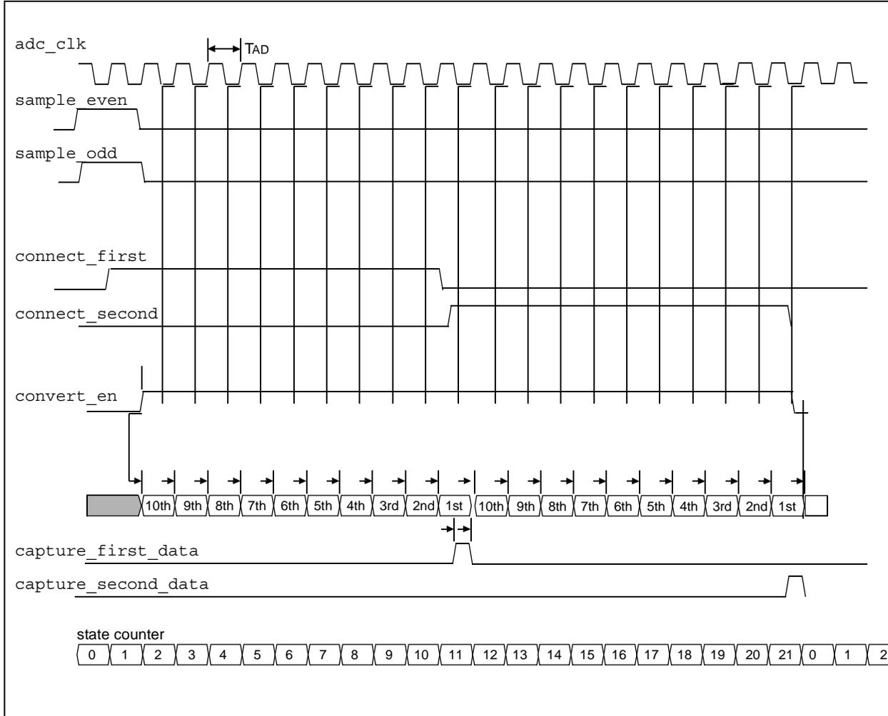
**FIGURE 16-4: DETAILED CONVERSION SEQUENCE TIMINGS, SEQSAMP = 1**
