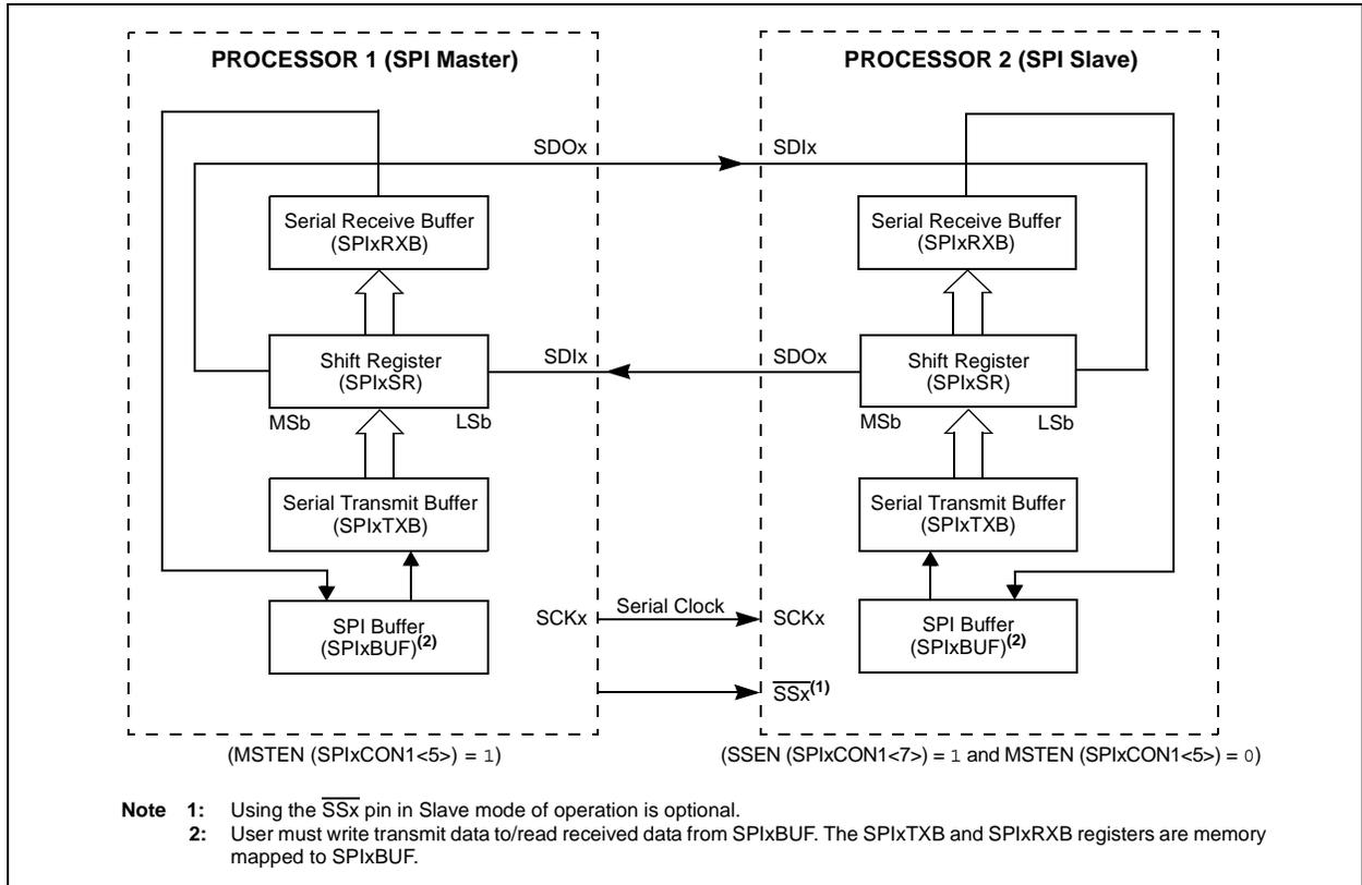
**FIGURE 13-3: SPI MASTER, FRAME MASTER CONNECTION DIAGRAM**
