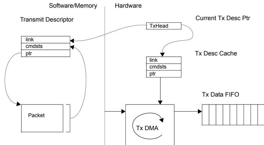
**Figure 5-4 Transmit Architecture**
