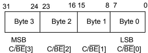
**Big Endian (CFG:BEM=1):** The byte orientation for receive and transmit data in system memory is as follows:
