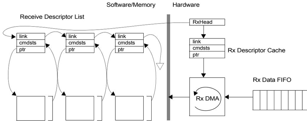
Figure 5-6 Receive Architecture
