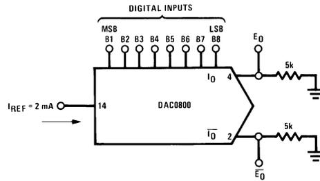
Pin numbers represent the PDIP package. The SOIC package pin numbers differ from that of the PDIP package.
