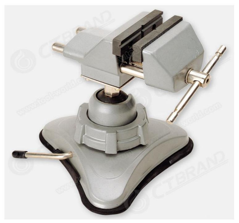
Aluminum workbench vise, desktop Jaw opening 70mm Jaw width 70mm Rotate 360° With Tilt adjustment
