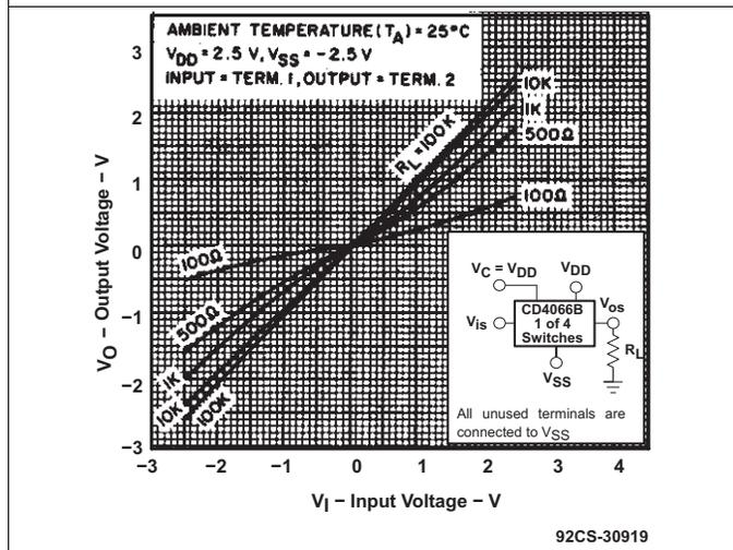
Figure 5. Typical ON Characteristics for 1 of 4 Channels
