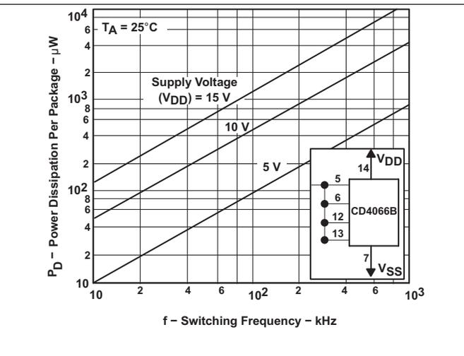
Figure 6. Power Dissipation per Package vs Switching Frequency
