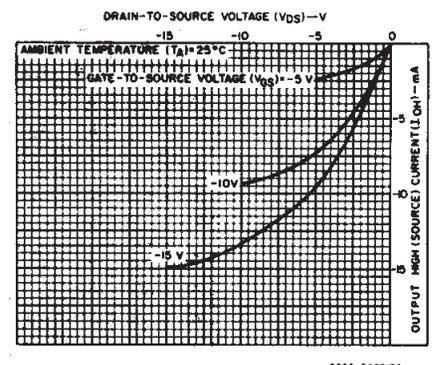
Fig. 6 - Minimum output high (source) current characteristics.
