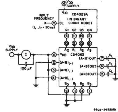
Fig. 12 - Dynamic power dissipation test circuit.
