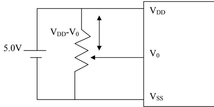
Where  $V_{DD}-V_0 = \text{LCD Driving voltage}$
