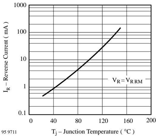
Figure 2. Max. Reverse Current vs. Junction Temperature
