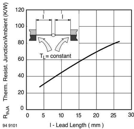
Figure 1. Typ. Thermal Resistance vs. Lead Length
