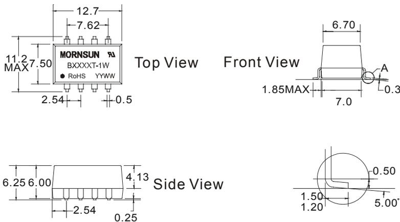
Note: All Pins on a 2.54mm pitch; all pin diameters are 0.50mm; all dimensions in mm.
