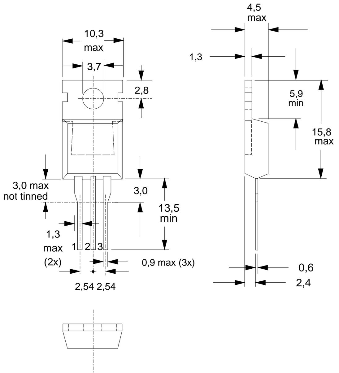
Fig. 13. SOT78 (TO220AB). pin 2 connected to mounting base.
