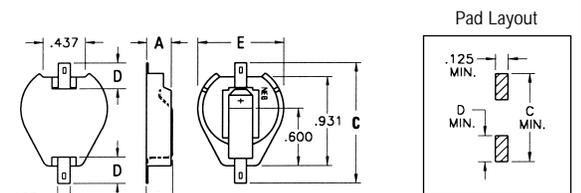
**MATERIAL:** Contacts: .015 Steel, Tin Plate Base: Nylon, Stanyl-46
