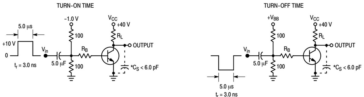
\*Total Shunt Capacitance of Test Jig and Connectors For PNP Test Circuits, Reverse All Voltage Polarities
