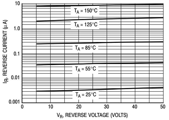
Figure 2. Leakage Current
