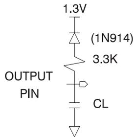
Note: 1.  $C_L = 100 \text{ pF}$  including jig capacitance, except for the -45 devices, where  $C_L = 30 \text{ pF}$ .
