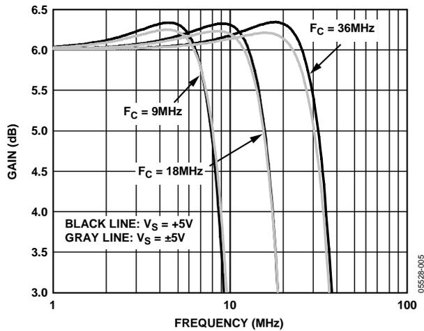
Figure 5. Frequency Response Flatness vs. Cutoff Frequency
