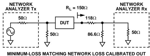
Figure 15. Basic Test Circuit for Swept Frequency Measurements
