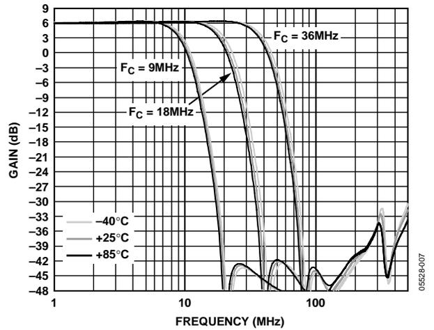
Figure 7. Frequency Response vs. Temperature and Cutoff Frequency
