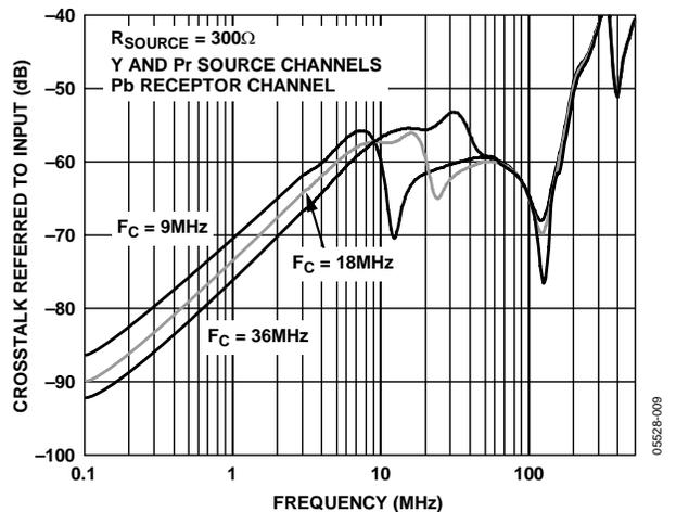
Figure 9. Channel-to-Channel Crosstalk vs. Frequency and Cutoff Frequency
