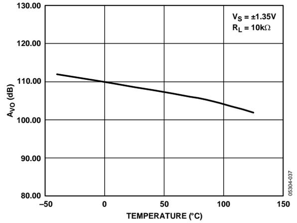
Figure 51. Large Signal Open-Loop Gain vs. Temperature
