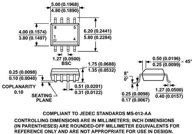
Figure 61. 8-Lead Standard Small Outline Package [SOIC\_N] Narrow Body (R-8)
