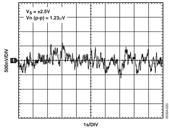
Figure 21. Low Frequency Noise (0.1 Hz to 10 Hz).
