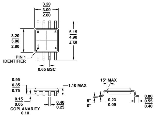
Figure 62. 8-Lead Mini Small Outline Package [MSOP] (RM-8)
