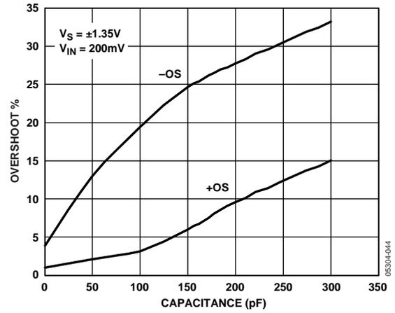
Figure 44. Small Signal Overshoot vs. Load Capacitance
