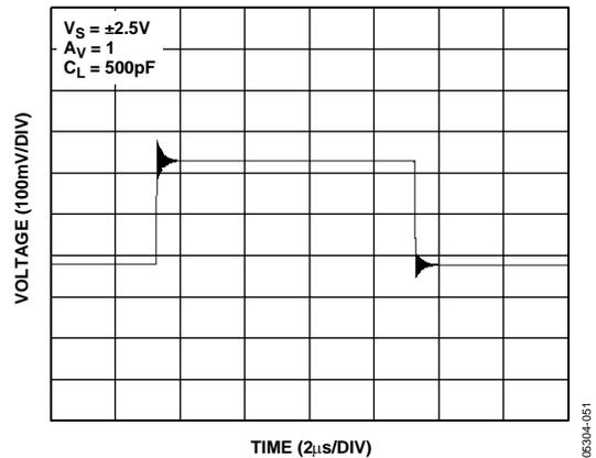
Figure 56. Driving Heavy Capacitive Loads Without Compensation
