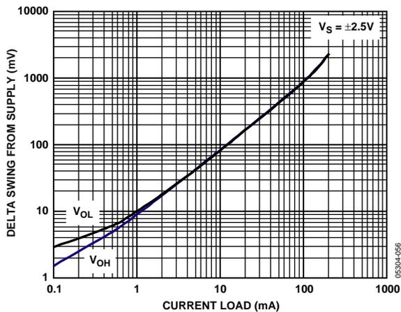
Figure 13. AD8656 Output Swing vs. Current Load
