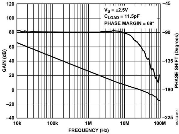
Figure 23. Open-Loop Gain and Phase vs. Frequency
