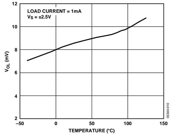
Figure 15. Output Voltage Swing Low vs. Temperature
