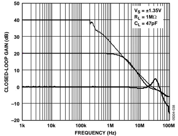
Figure 52. Closed-Loop Gain vs. Frequency
