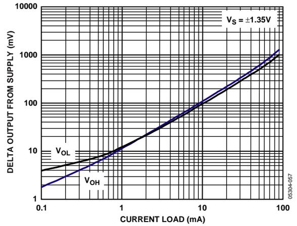
Figure 38. AD8656 Output Swing vs. Current Load
