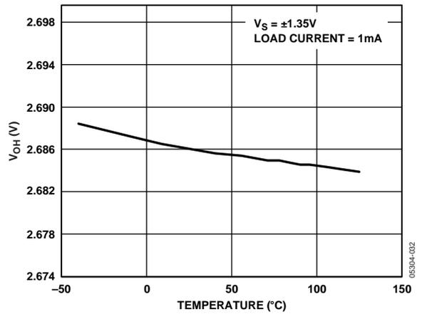
Figure 39. Output Voltage Swing High vs. Temperature
