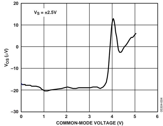
Figure 8. Input Offset Voltage vs. Common-Mode Voltage
