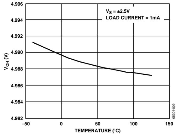
Figure 14. Output Voltage Swing High vs. Temperature
