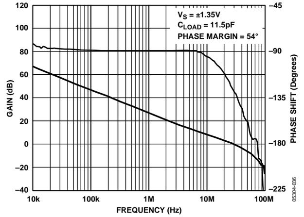
Figure 50. Open-Loop Gain and Phase vs. Frequency
