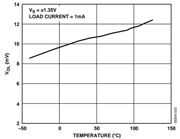
Figure 40. Output Voltage Swing Low vs. Temperature
