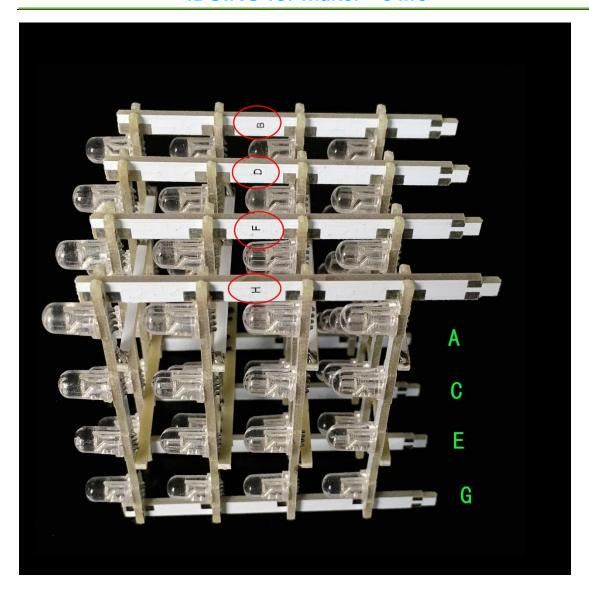
Then plug the plate into the base board and solder:
