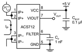
Application 1. The ACS712 outputs an analog signal,  $V_{OUT}$ , that varies linearly with the uni- or bi-directional AC or DC primary sensed current,  $I_P$ , within the range specified.  $C_F$  is recommended for noise management, with values that depend on the application.
