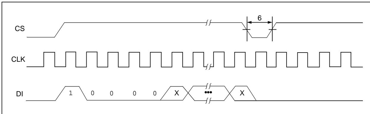
**FIGURE 2-4: WRITE TIMING**
