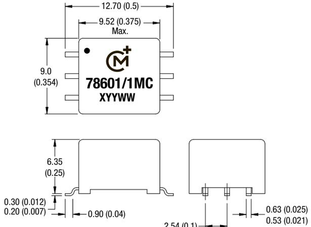
Unless otherwise stated all dimensions in mm (inches)  $\pm 0.25$  (0.01). All pins on a 2.54 (0.1) pitch and within  $\pm 0.25$  (0.01) of true position.
