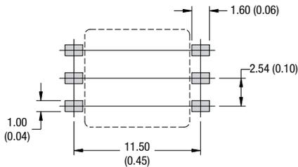
Unless otherwise stated all dimensions in mm (inches)  $\pm 0.25$  (0.01). All pins on a 2.54 (0.1) pitch and within  $\pm 0.25$  (0.01) of true position.
