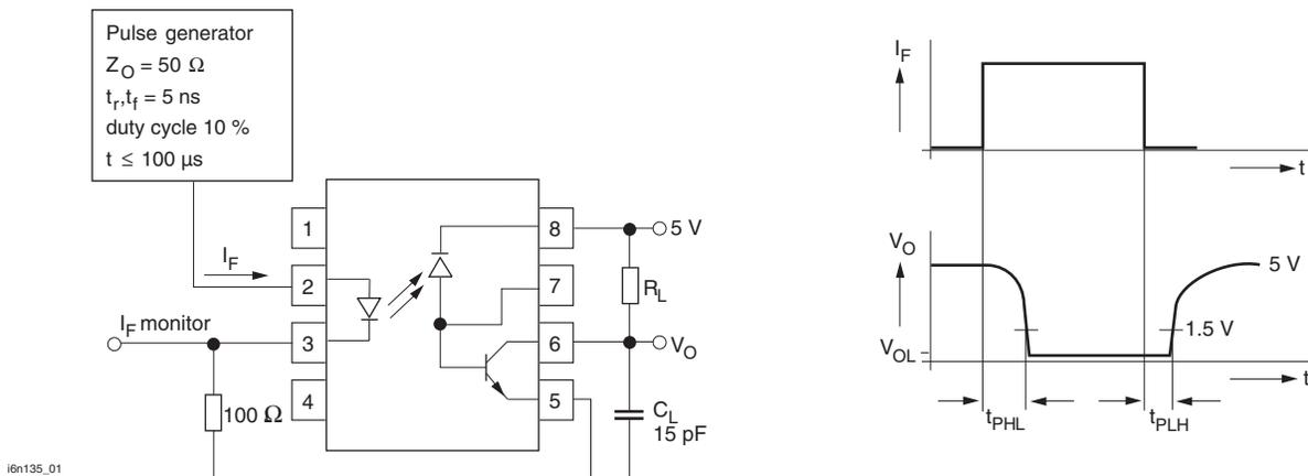
Fig. 10 - Switching Times
