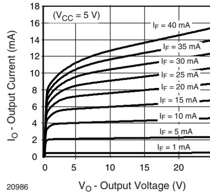
Fig. 4 - Output Current vs. Output Voltage
