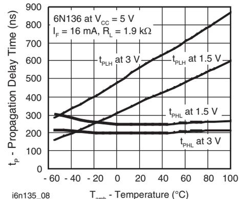
Fig. 6 - Propagation Delay vs. Ambient Temperature
