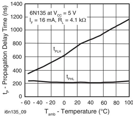
Fig. 7 - Propagation Delay vs. Ambient Temperature
