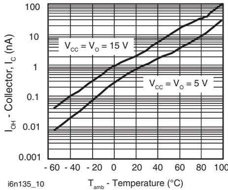
Fig. 8 - Logic High Output Current vs. Temperature
