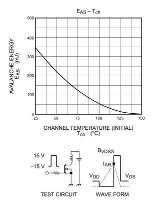
$\begin{aligned} &R_G = 25~\Omega\\ &V_{DD} = 90~V,~L = 16.8mH \end{aligned} \qquad \text{EAS} = \frac{1}{2} \cdot L \cdot I^2 \cdot \left( \frac{BVDSS}{BVDSS - VDD} \right)$
