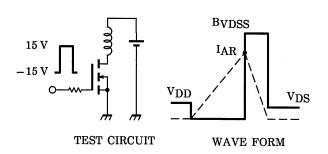
$$\begin{aligned} &RG = 25 \ \Omega \\ &V_{DD} = 90 \ V, \ L = 12 \ mH \end{aligned} \qquad EAS = \frac{1}{2} \cdot L \cdot I^2 \cdot \left( \frac{BVDSS}{BVDSS - VDD} \right)$$
