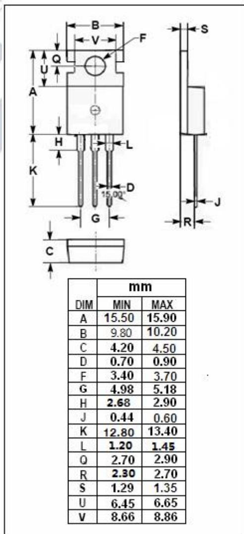
**isc Silicon NPN Power Transistors****2SD1237****ELECTRICAL CHARACTERISTICS****T<sub>c</sub>=25°C unless otherwise specified**
