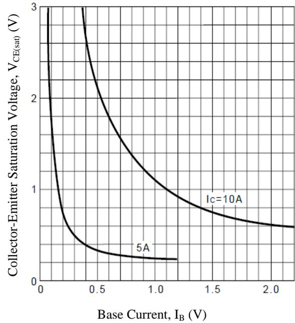
Figure 4. Collector-Emitter Saturation Voltage vs. Base Current
