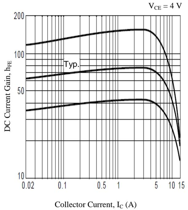
Figure 6. DC Current Gain Variation vs. Collector Current
