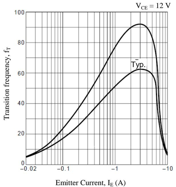
Figure 8. Transition Frequency vs. Emitter Current
