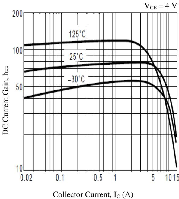
Figure 7. DC Current Gain vs. Collector Current
