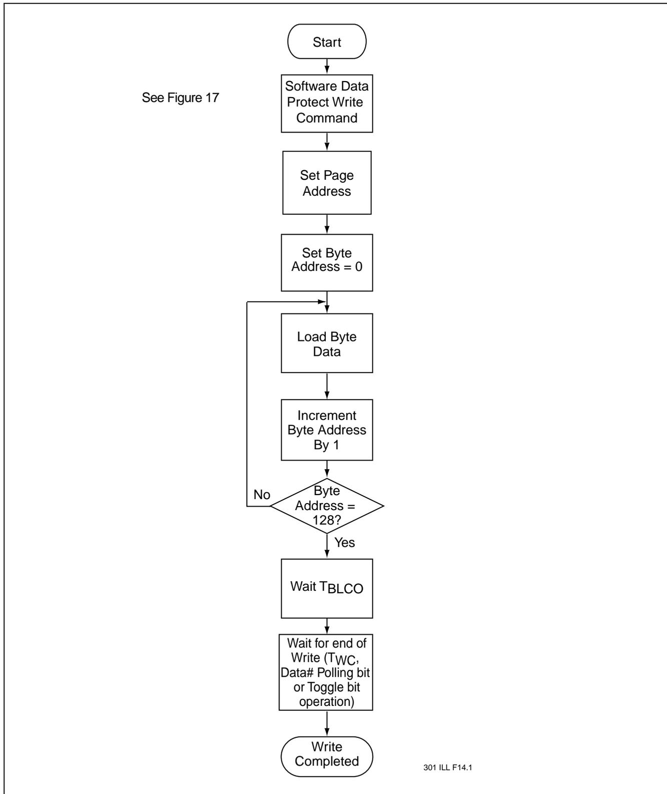
FIGURE 15: WRITE ALGORITHM
