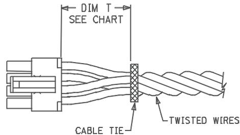
The "T" dimension defines a "free" length of wire, or a length of wire that is not subject to significant bias by external factors such as a wire tie, wire twisting, or other means of bending or deforming of the wires that repositions them from their natural relaxed state or location where they enter the housing. Wires are to be dressed in such a manner to allow the terminals to float freely in the pocket.
